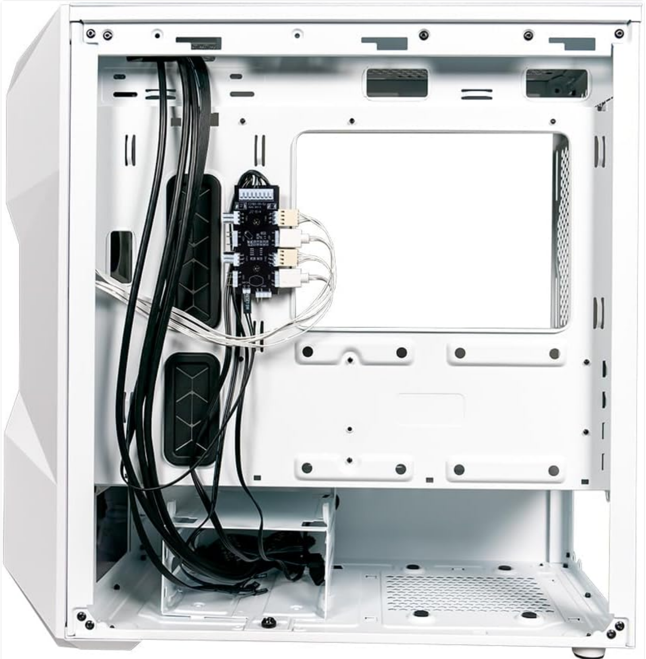
Figure 4.2: Rear interior view of the case, showing the cable management area and the integrated PWM/ARGB hub.
