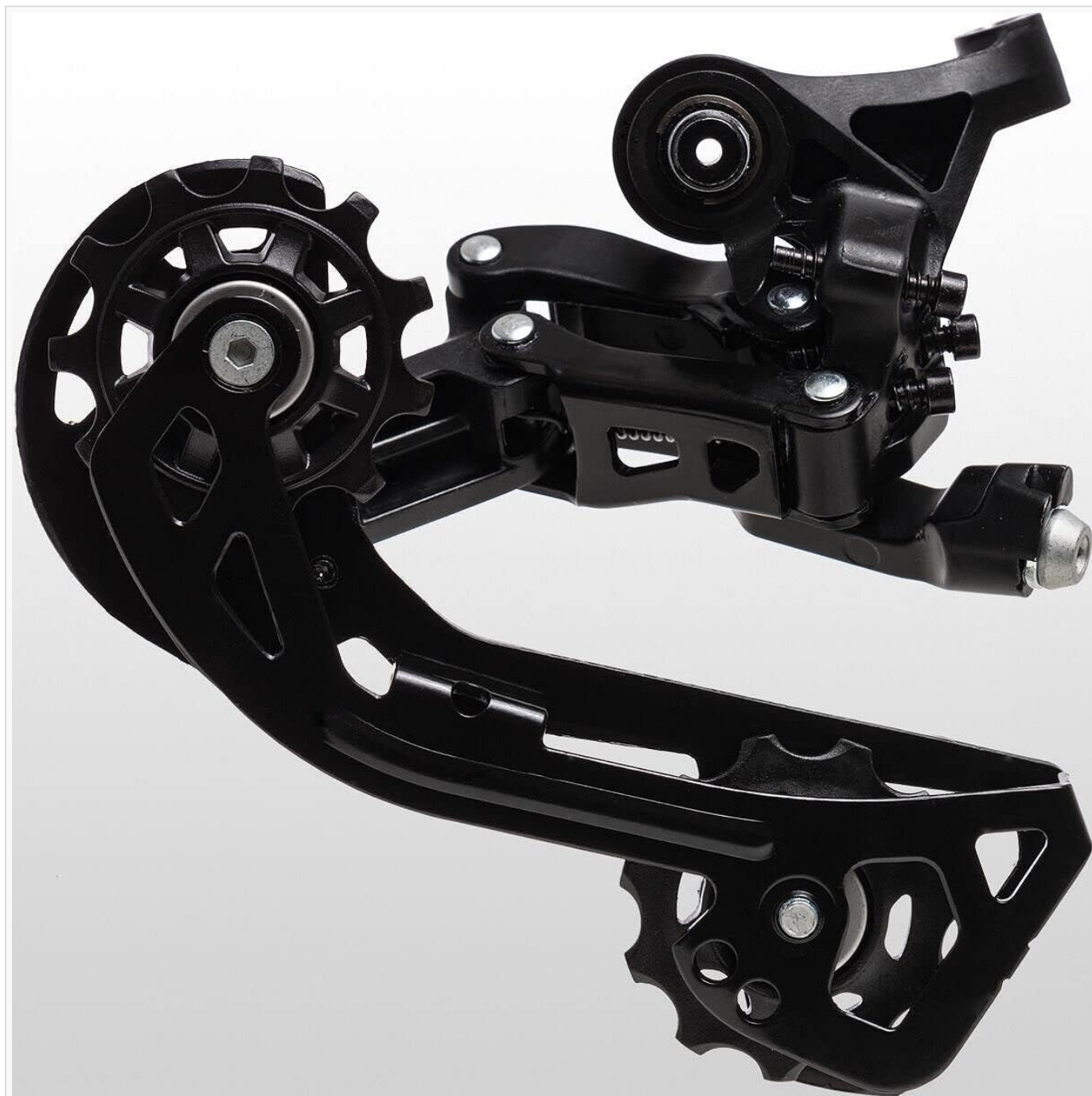
Figure 2: Side view of the derailleur, highlighting the medium cage and jockey wheels.
