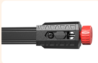
Figure 6.1: The integrated belt tensioner simplifies maintenance and improves print quality.
