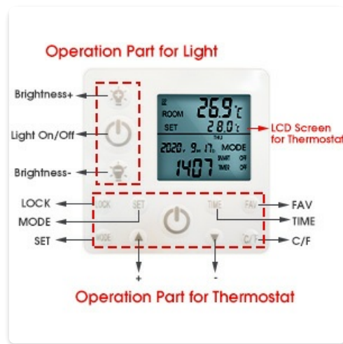
Image 5.1: Diagram of the remote control, detailing buttons for light operation (Brightness+, Light On/Off, Brightness-) and thermostat operation (LOCK, MODE, SET, TIME, FAV, C/F, Power, Temperature Up/Down).
