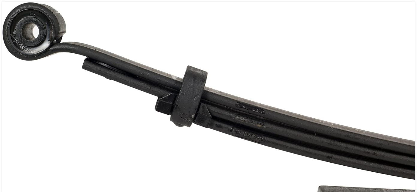
Figure 2.3: Close-up view of the front eyelet and leaf pack of the Dorman 43-1851 Rear Leaf Spring, highlighting the robust construction.
