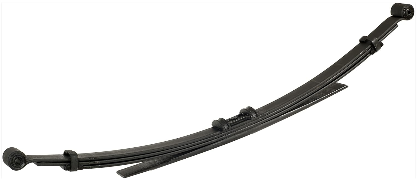
Figure 2.1: The Dorman 43-1851 Rear Leaf Spring, a direct replacement component for vehicle suspension systems.
