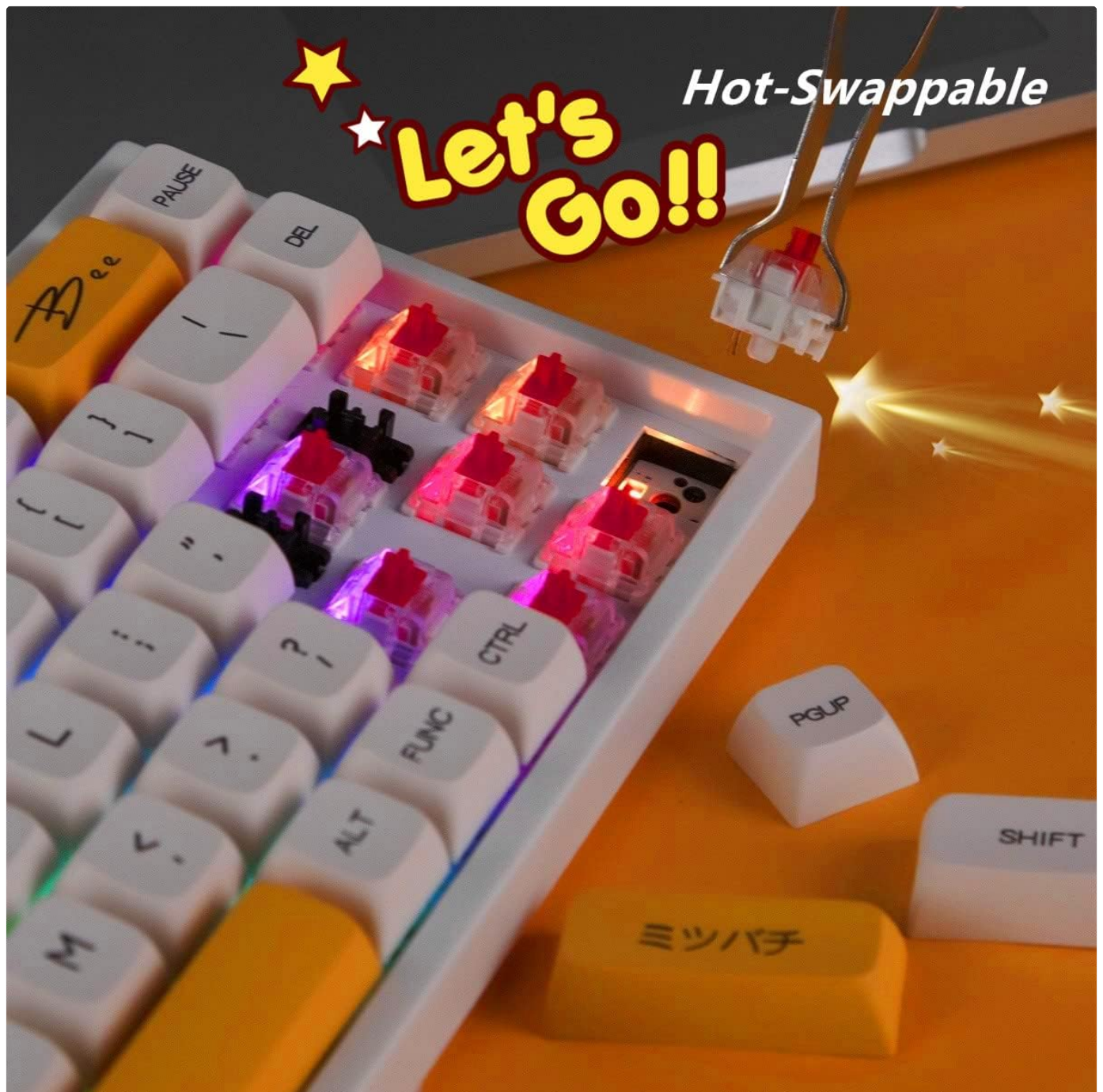
Image: A close-up view demonstrating the hot-swappable feature, with a switch puller removing a Gateron switch from the keyboard.
