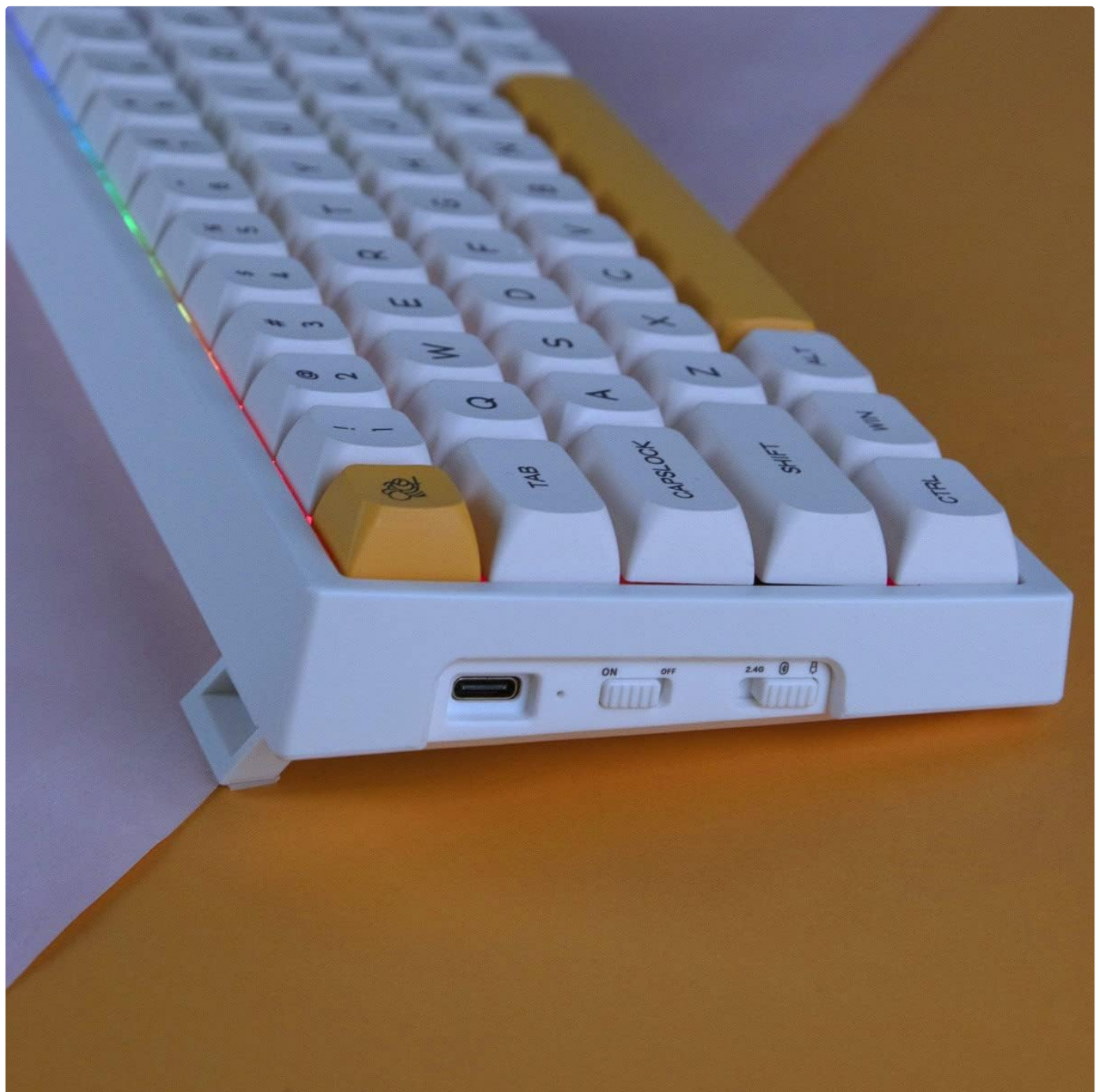
Image: Side view of the keyboard highlighting the USB Type-C port and the physical switches for connectivity modes (ON/OFF, 2.4G).
