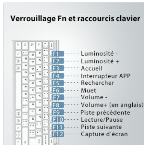
Figure 7: Diagram detailing the function key shortcuts available on the iClever BK10 keyboard.
