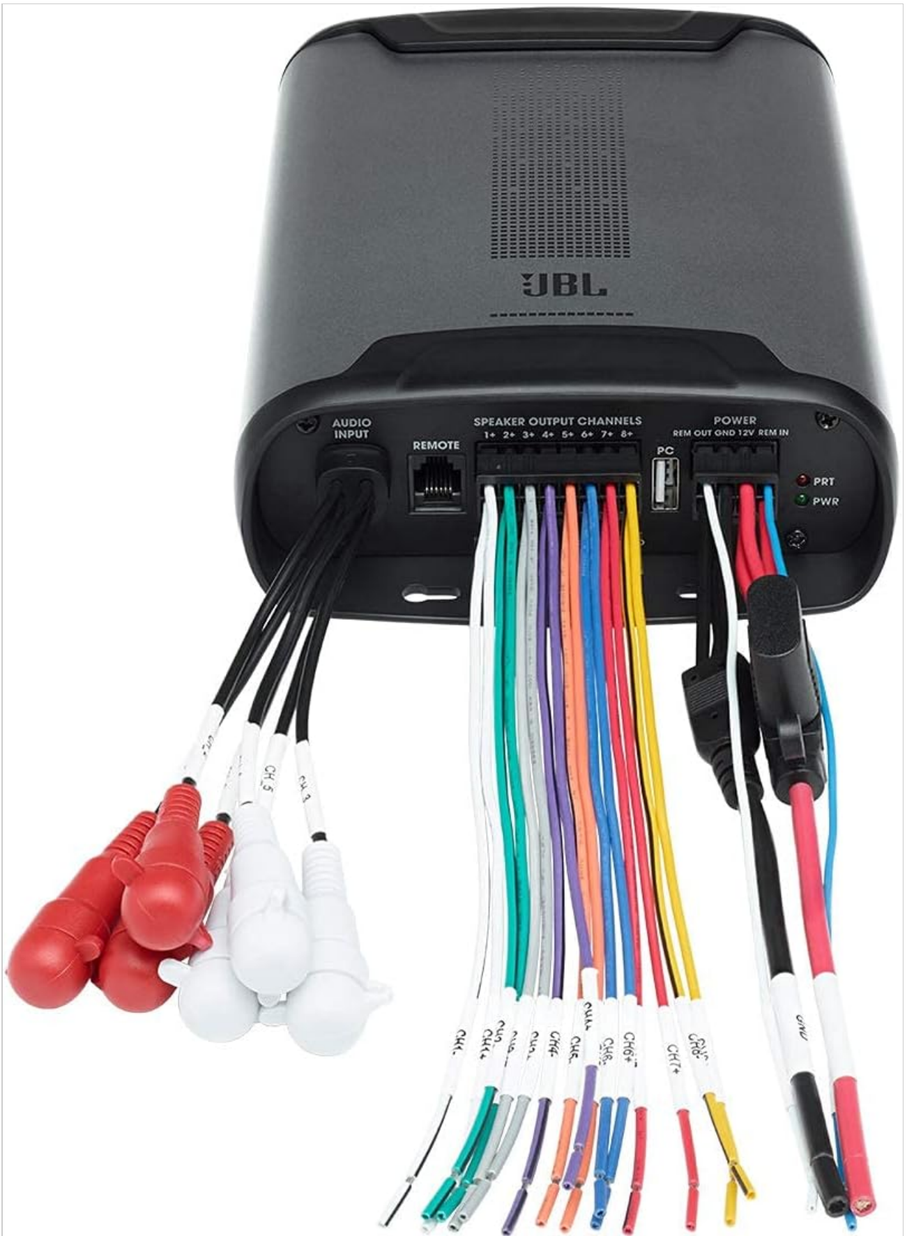
Figure 3.3: The JBL DSP4086 amplifier with all necessary cables connected, illustrating a complete wiring setup. This provides a visual guide for how the amplifier should appear once fully wired.
