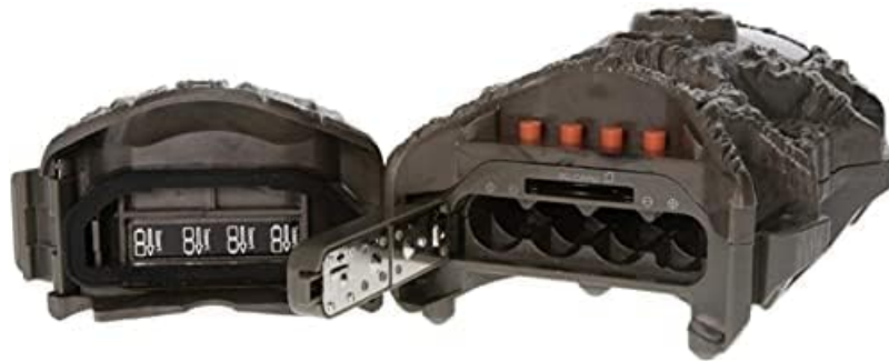
Figure 3: Interior view of the camera, revealing the battery compartment for 8 AA batteries and the SD card slot.
