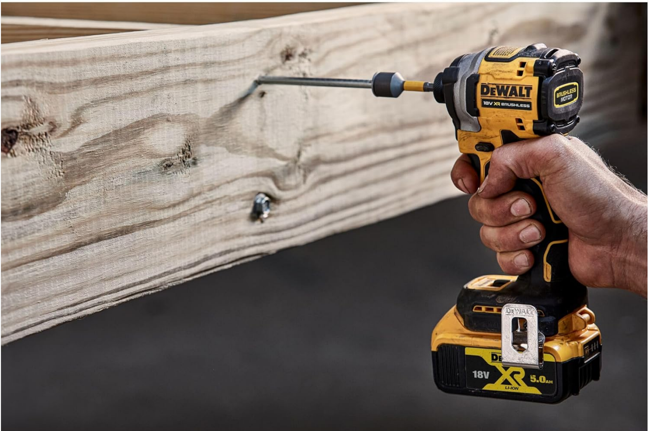
Figure 8: The impact driver driving a long screw into a wooden beam.
