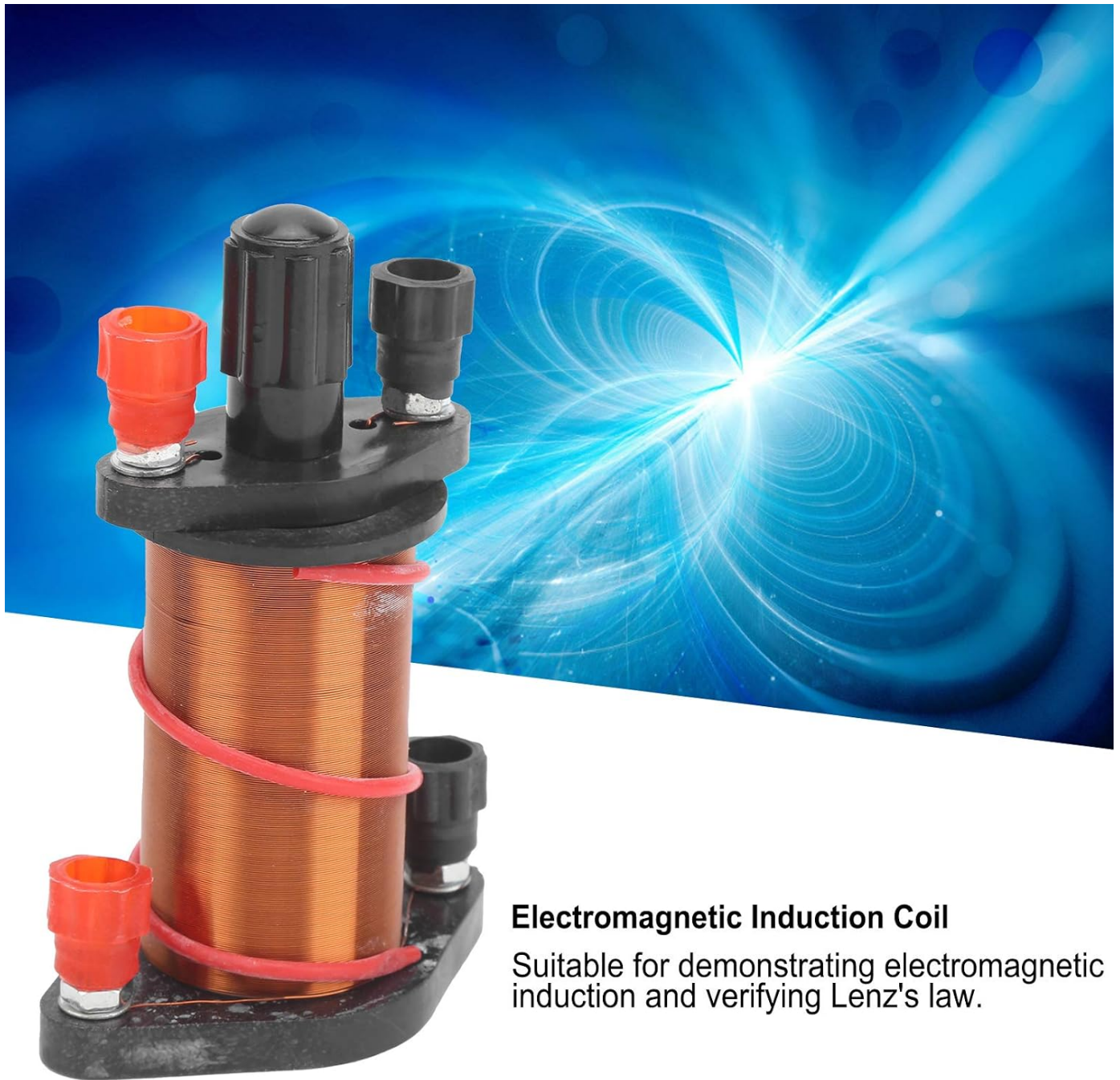
Image 1.1: The Electromagnetic Induction Coil Kit, suitable for demonstrating electromagnetic induction and verifying Lenz's law.
