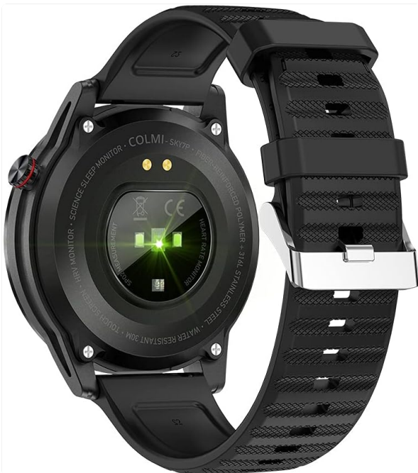
Figure 3.3: Rear view of the smart watch, displaying the optical heart rate sensor and magnetic charging pins. The model name 'COLMI SKY7P' is visible.
