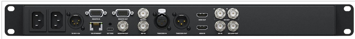
Figure 3: Rear panel connections including SDI, HDMI, Ethernet, and power inputs.
