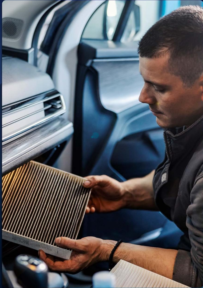
Image 3: Detailed view highlighting the activated carbon core for odor neutralization and the high-density pleated filter media designed for efficient particle capture.
