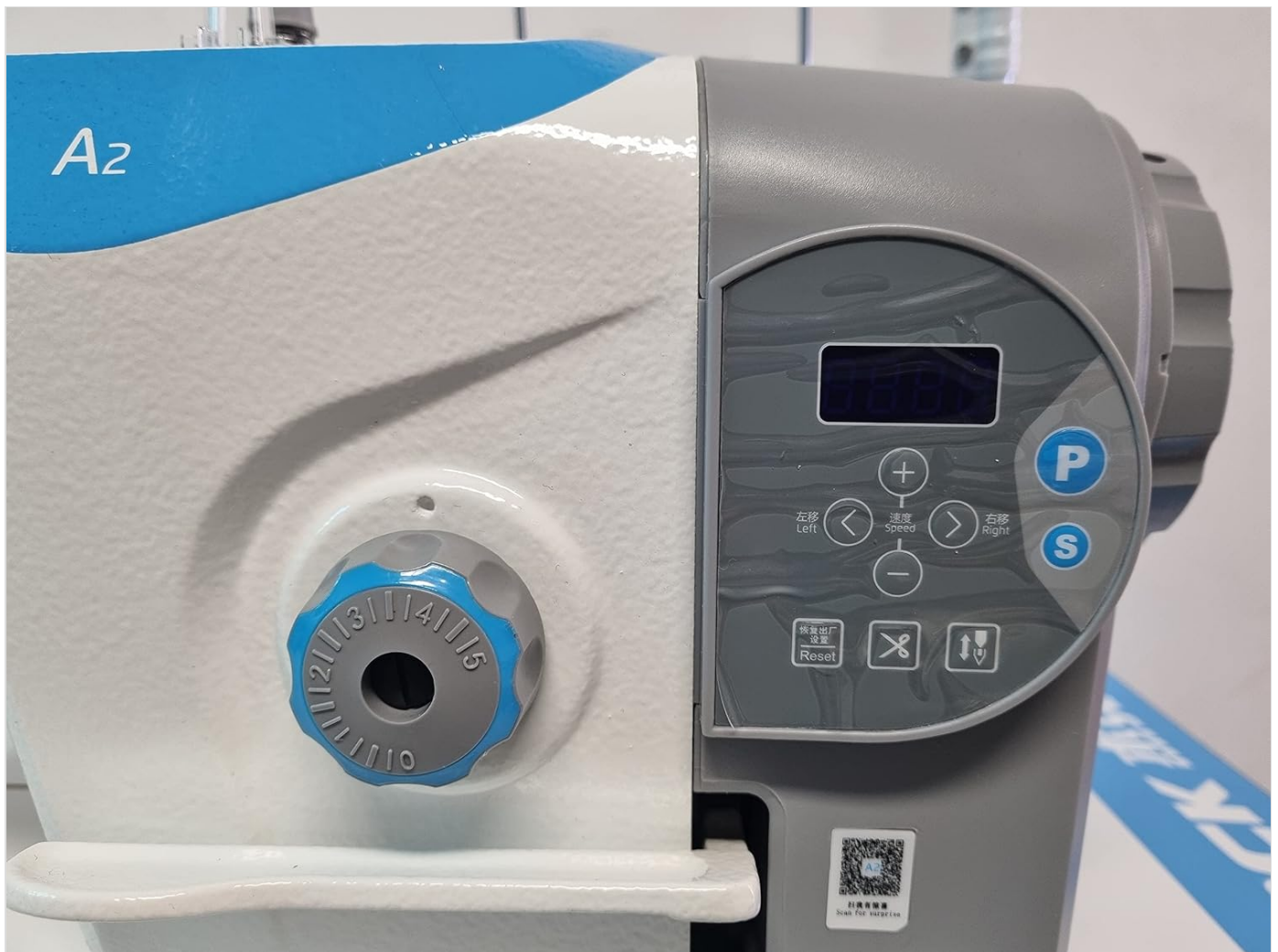
Image: A close-up of the digital control panel, showing speed adjustment buttons and other function controls.
