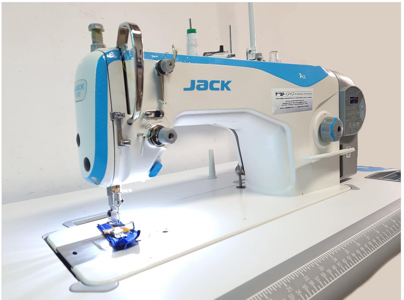
Image: Front view of the Konsew JACK A2 machine head, highlighting the needle area and presser foot.
