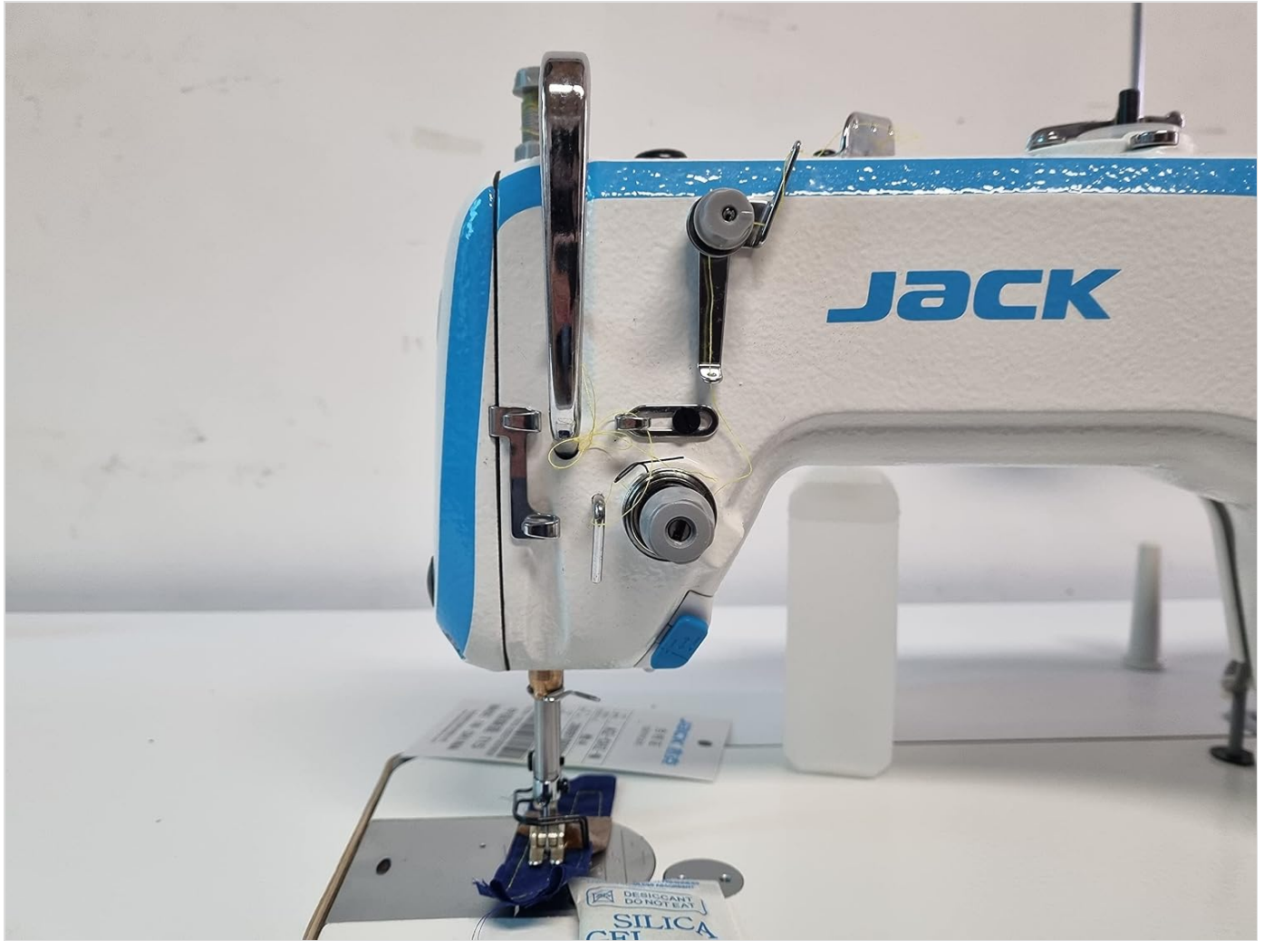
Image: A detailed view of the upper threading path, showing the thread guides and tension assembly.
