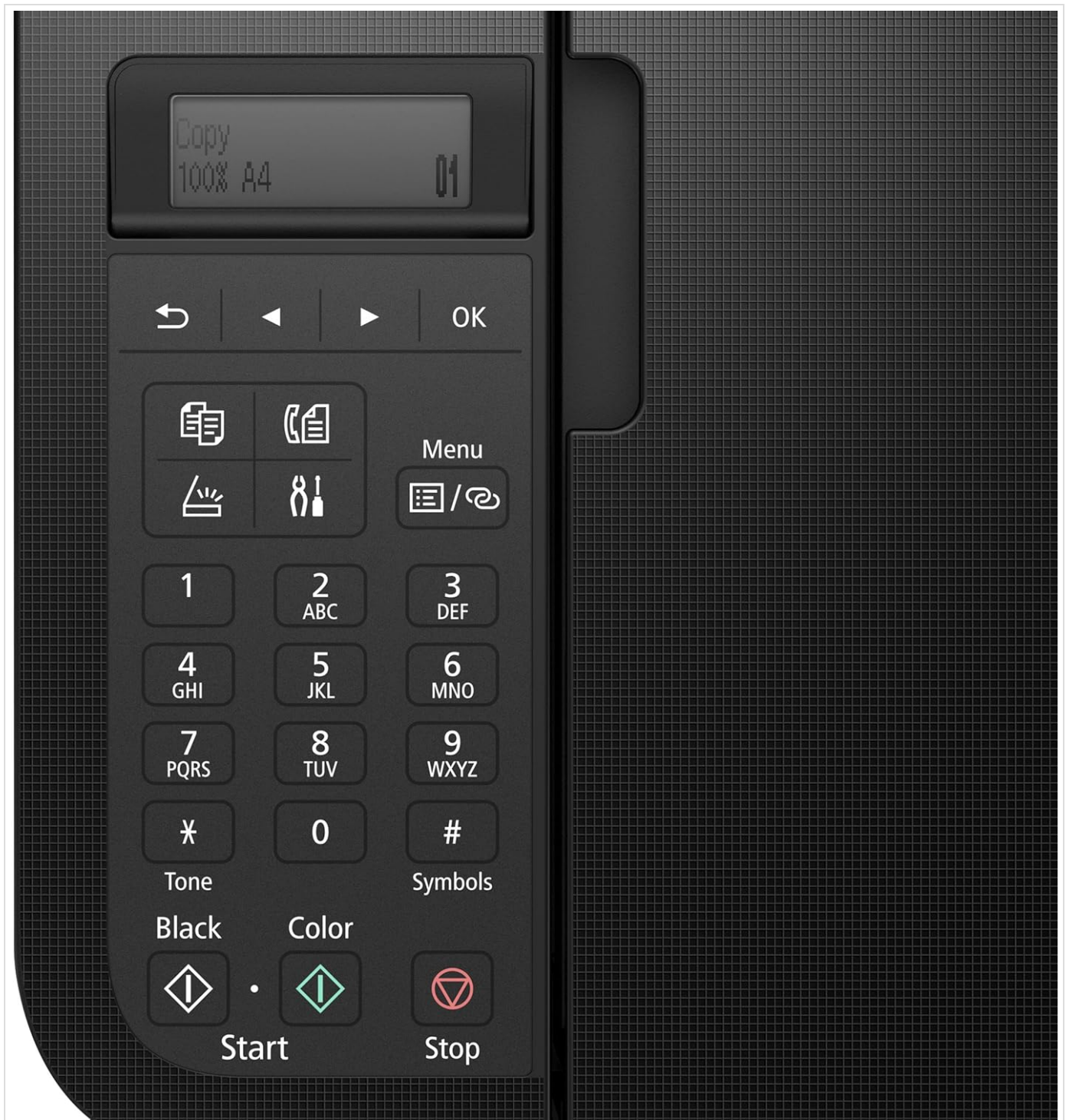
Image 7: A detailed view of the Canon PIXMA TR4720's control panel, showing the 2-Line LCD display, numeric keypad, and function buttons for easy operation.
