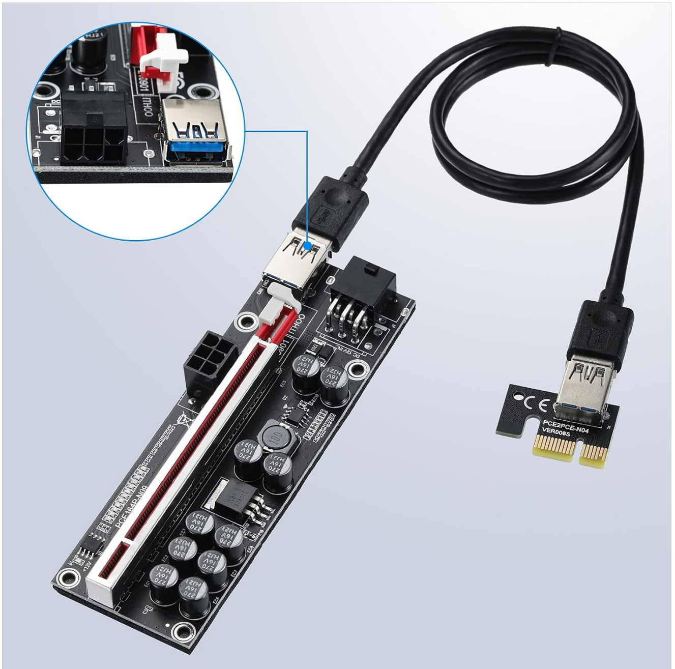
Figure 6.1: USB 3.0 cable connection. This image illustrates how to connect the USB 3.0 cable between the PCI-E 1X plug-in card and the PCI-E 16X main riser card.
