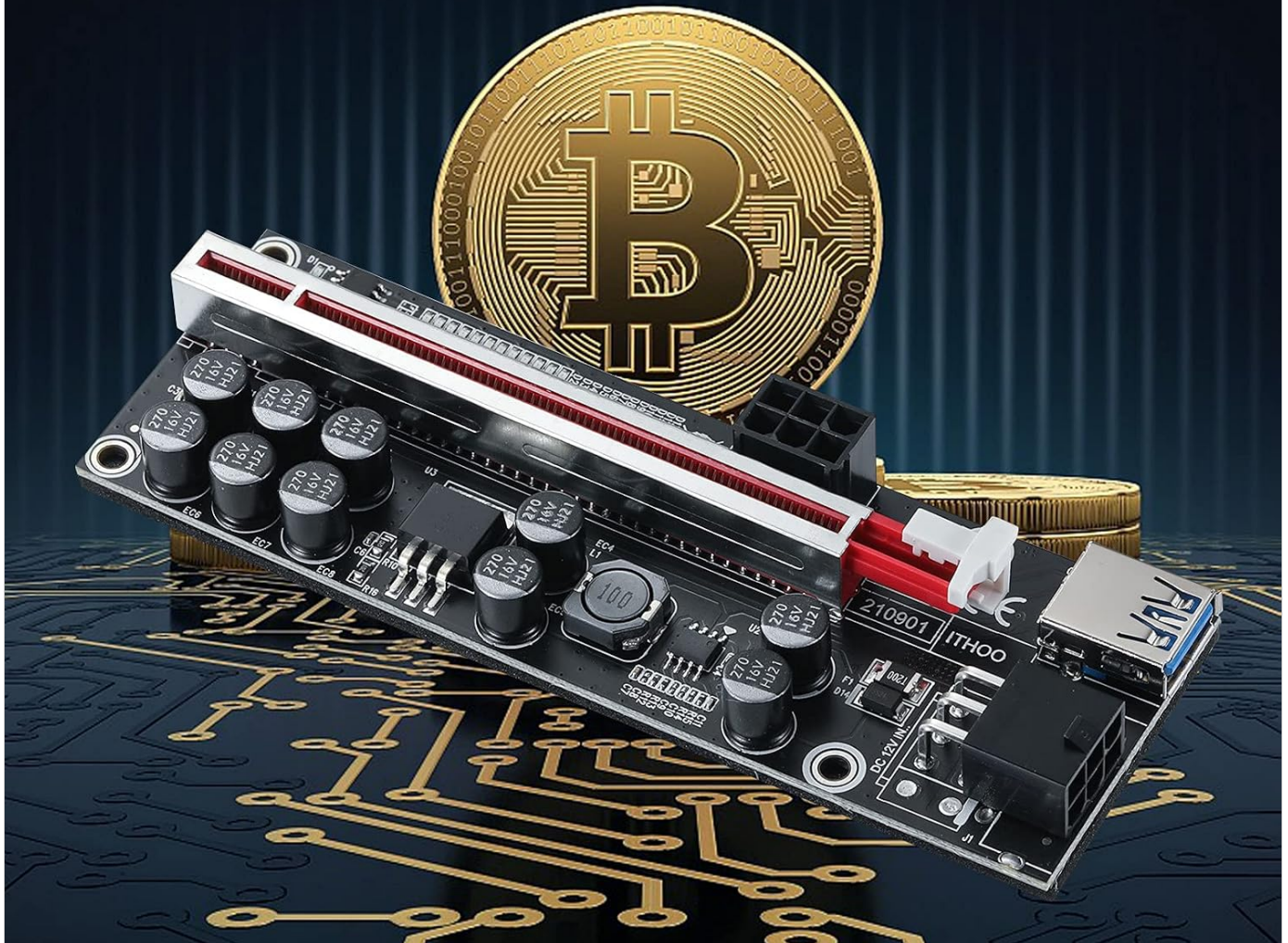
Figure 2.2: Detailed view of the riser card components. This image highlights the 10 solid capacitors for power stability, power inductance, dual 6PIN power supply port, LED power indicator, and the USB 3.0 port for connection to the PCI-E 1X plug-in card.
