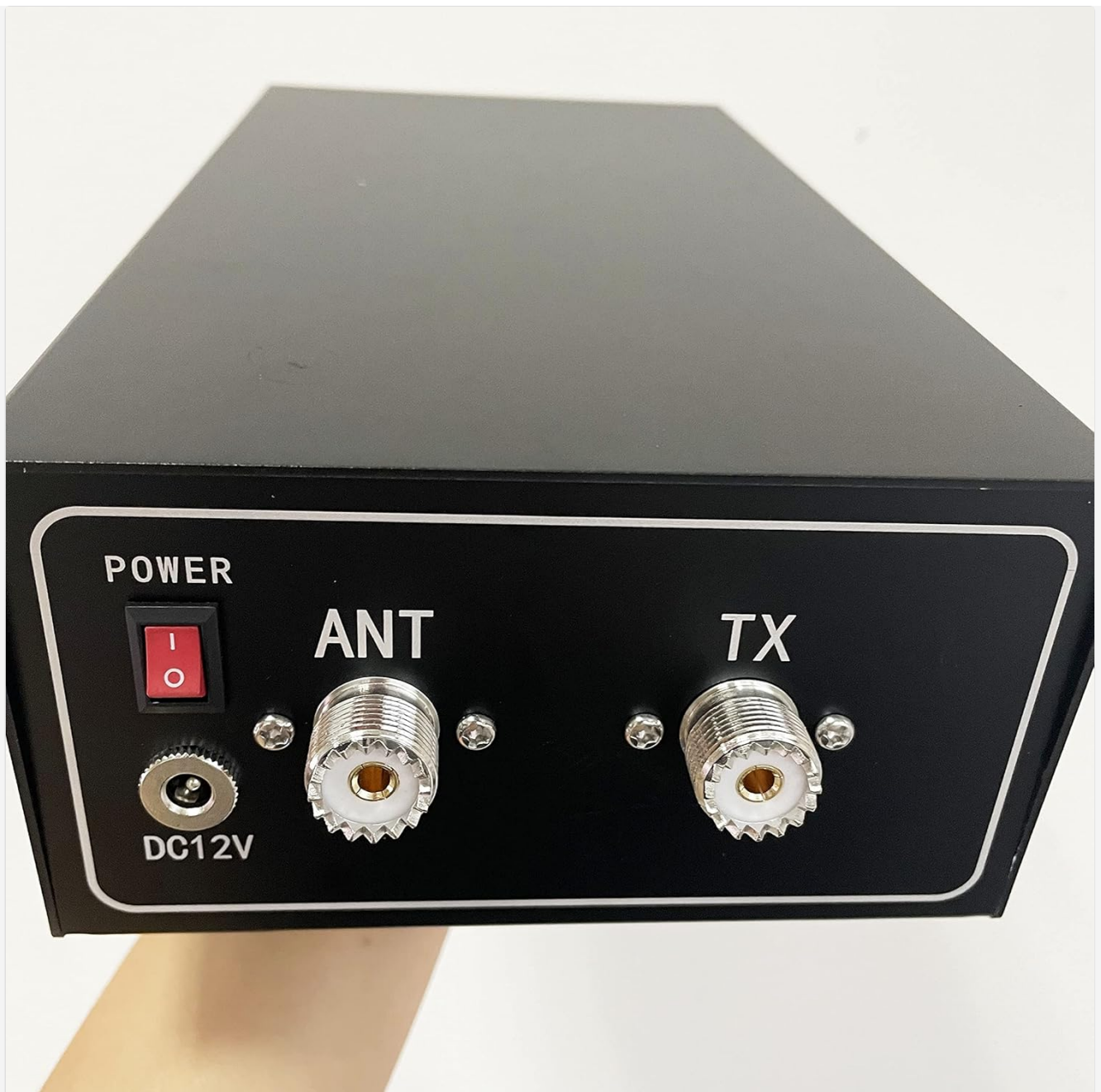
Figure 4: Close-up of the rear panel showing the DC12V input, power switch, ANT, and TX connectors.
