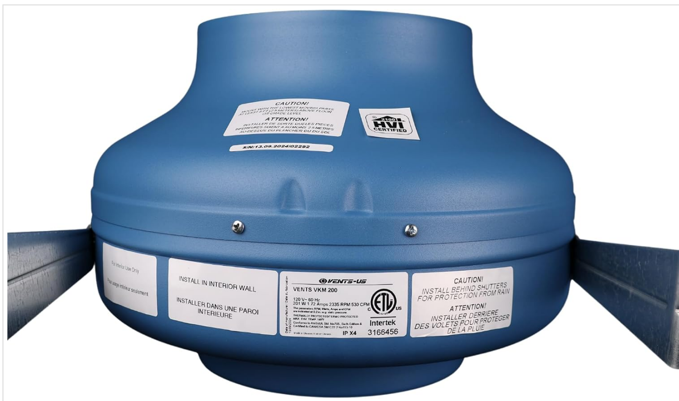
Image 4: Bottom view of the VKM 200 fan, showing the labels with installation instructions and certifications. Note the "Install in Interior Wall" and "Install Behind Shutters for Protection from Rain" cautions.
