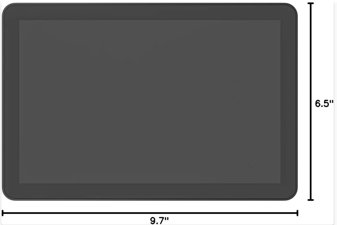
Figure 7.1: Diagram illustrating the physical dimensions of the Logitech Tap Scheduler.
