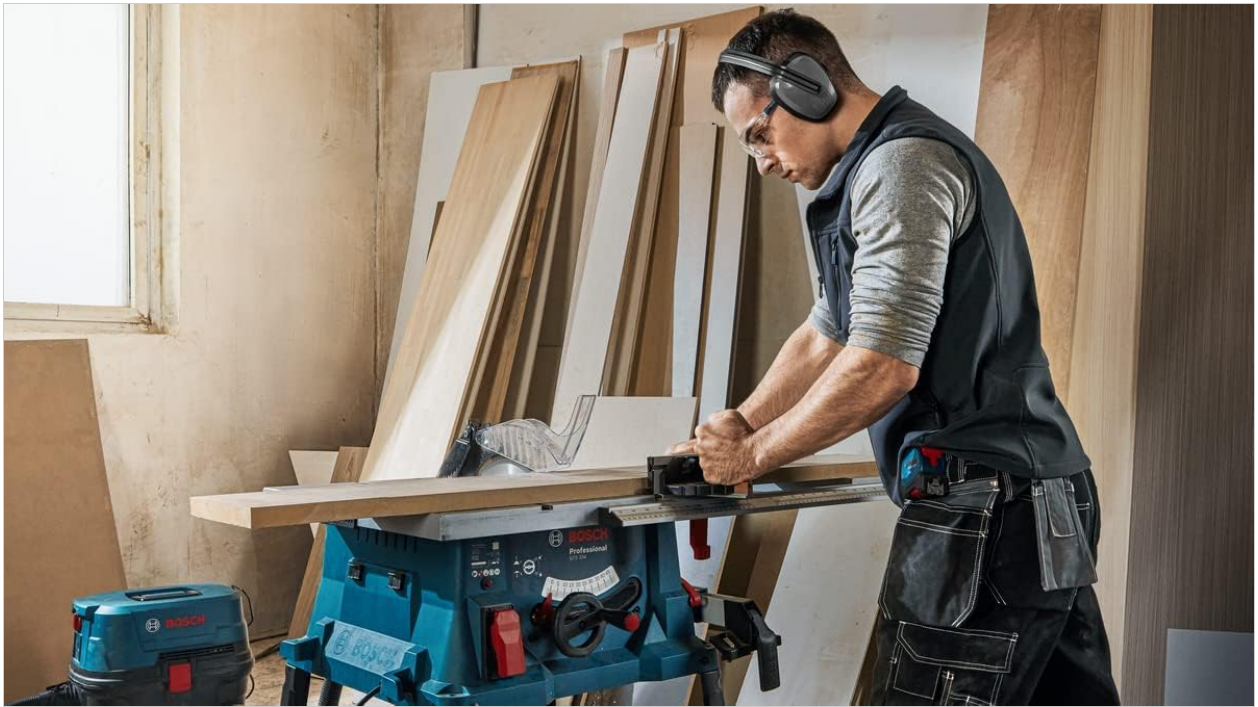
Image: A user performing a cross-cut on the Bosch GTS 254 table saw, utilizing the miter gauge for accurate cuts.
