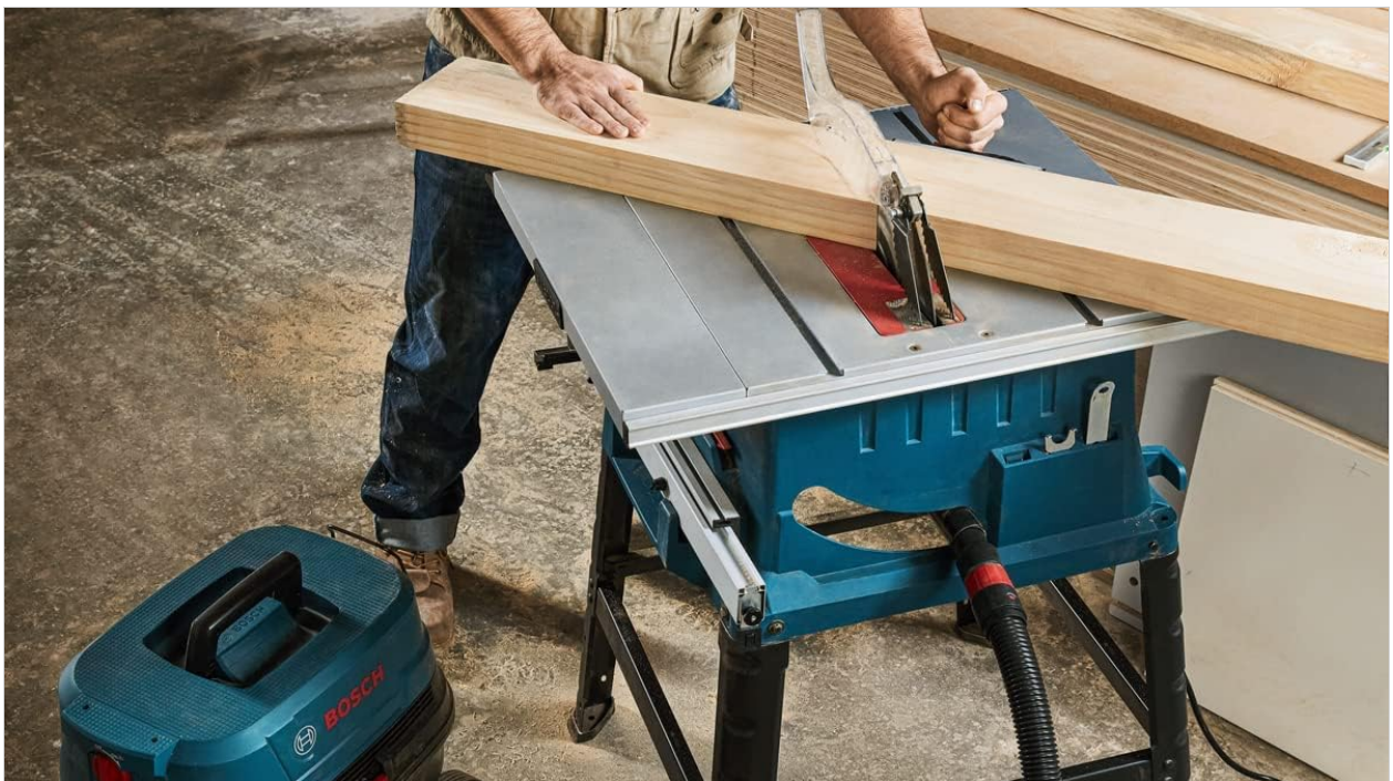
Image: A user performing a rip cut on the Bosch GTS 254 table saw, demonstrating the use of the rip fence and proper hand placement.
