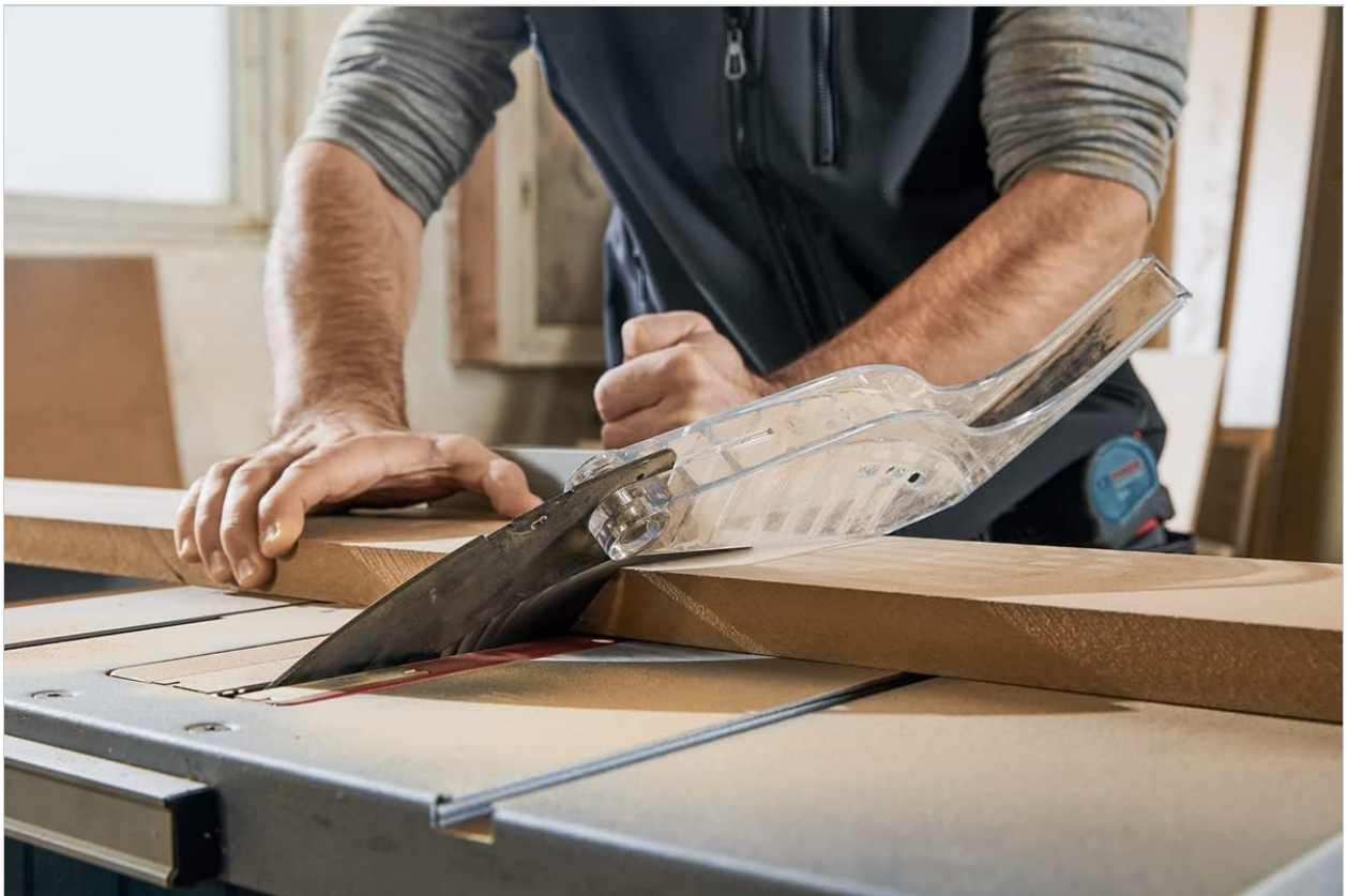
Image: Close-up view of the Bosch GTS 254 table saw blade and transparent guard during operation, showing the cutting action.
