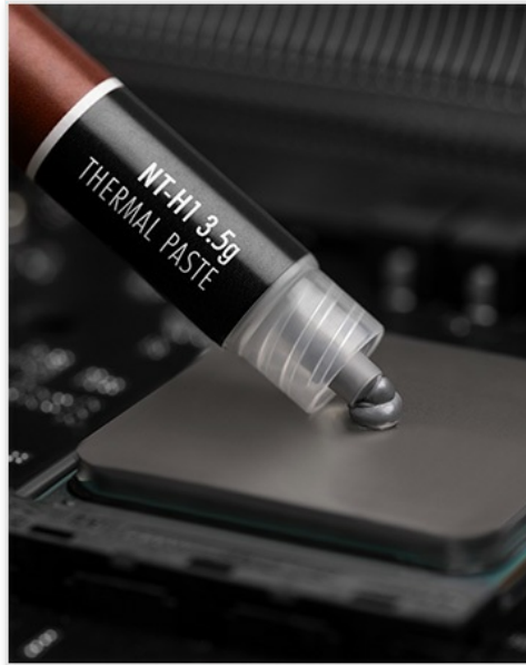
Image 3.2: Proper application of NT-H1 thermal compound to the CPU.
