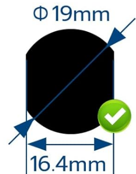
Figure 5.1: Choose the Right Latch Size. This diagram provides guidance on selecting the appropriate latch size for your cabinet, detailing the lock shaft dimensions and required cabinet thickness (up to 30mm).
