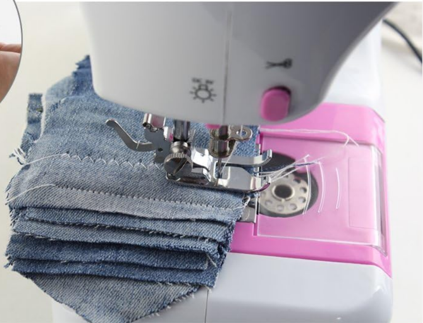
Figure 3: Close-up view of the bobbin area and needle plate, showing the improved hook quality.
