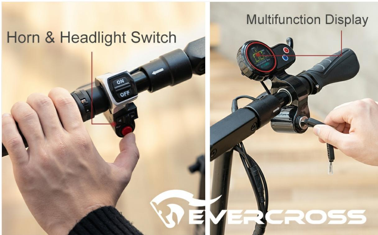
This image illustrates the instrument display mounted on an electric scooter handlebar, showing the key inserted into the ignition and the multifunction display in operation. It also highlights the horn and headlight switch on the left handlebar.
