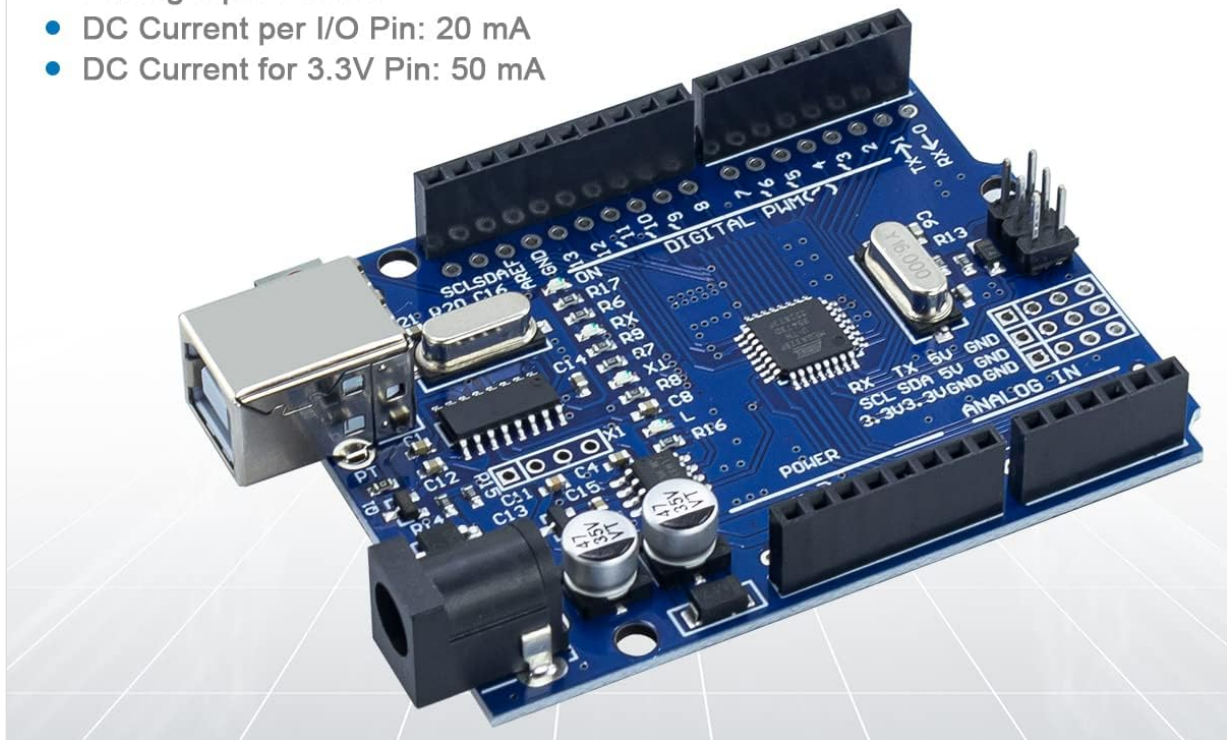
Image 3.1: The LAFVIN R3 CH340 board, detailing its components and specifications.
