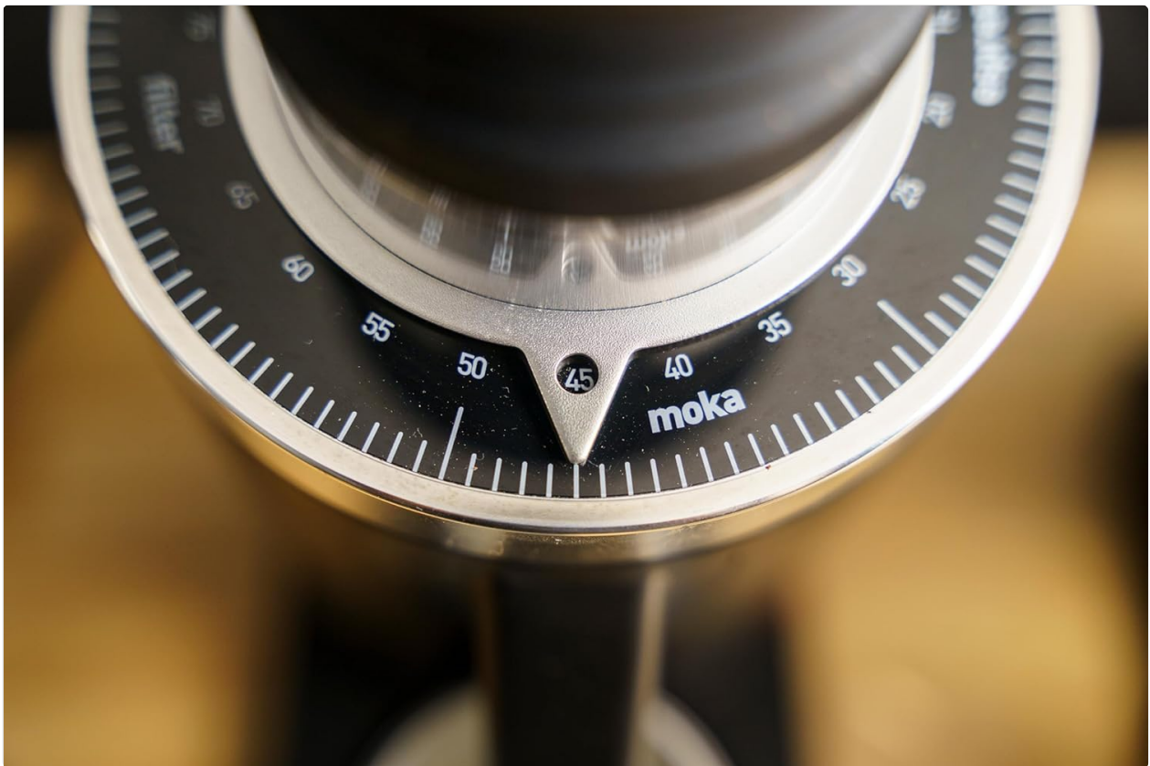
Figure 2: Stepless grind adjustment dial.
