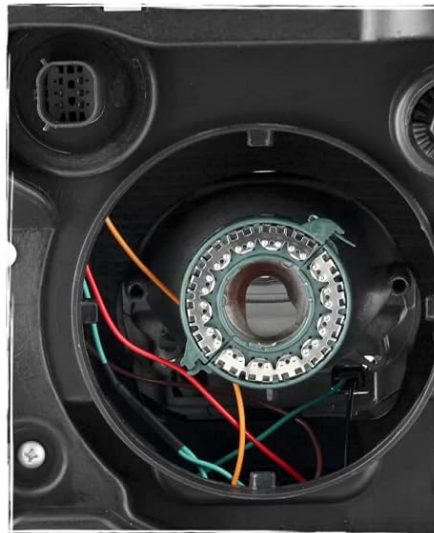
Image 2: Rear view of the headlight assembly, illustrating electrical connections and bulb access points.
