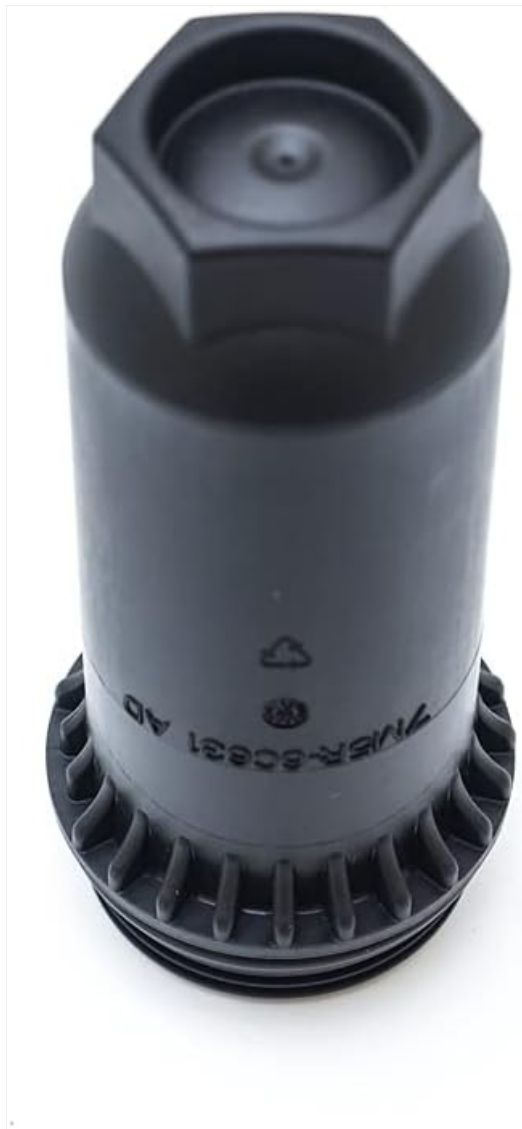
Image 5: Top-down view of the oil filter housing cap, showing the hexagonal tightening point and the ribbed grip for handling.
