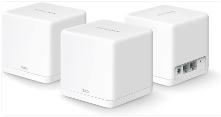
Three Mercusys Halo H30G units, with one unit rotated to show the rear ports (power, Ethernet).
