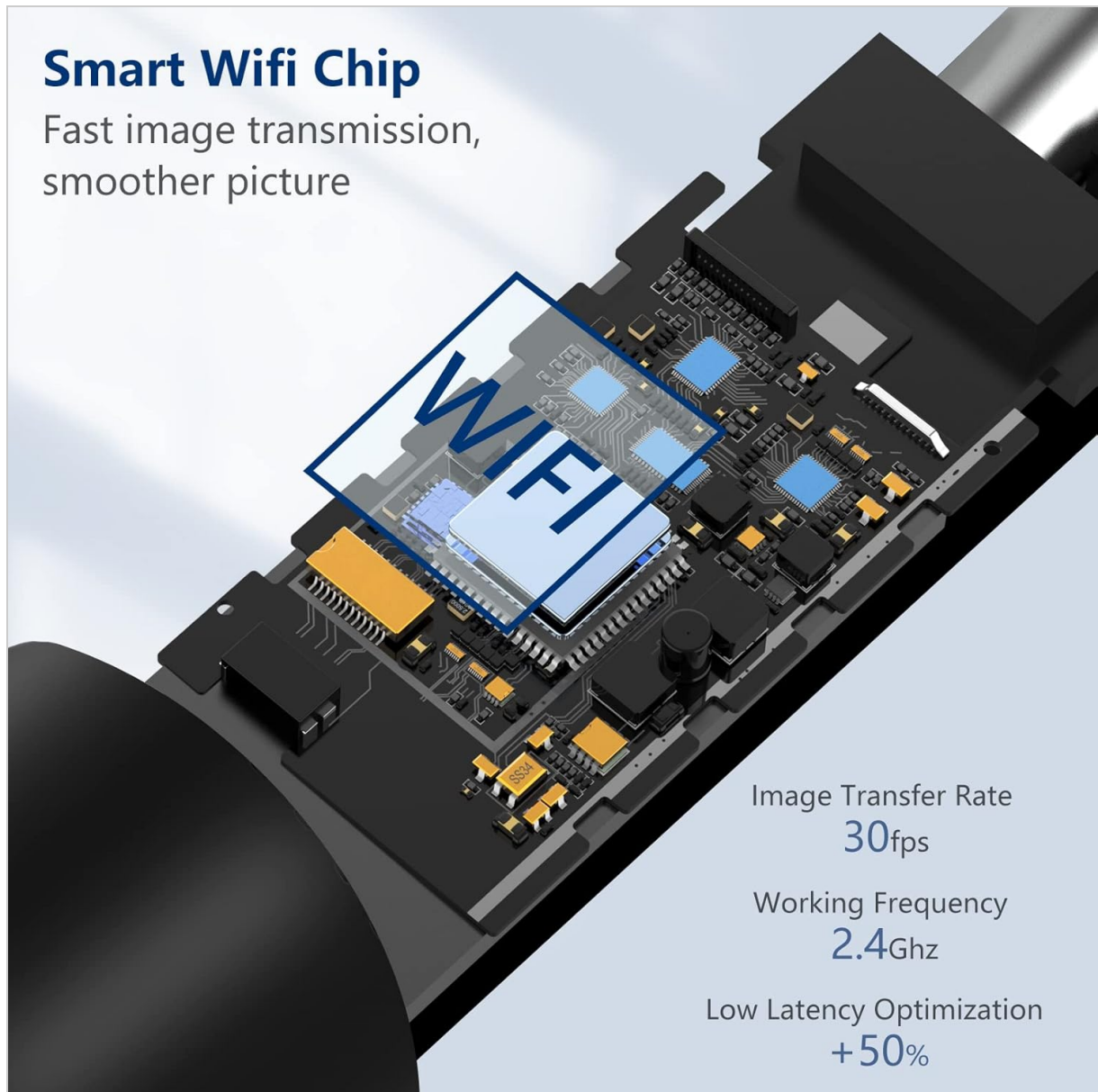
Image 5.2: The integrated Smart WiFi Chip ensures fast and smooth image transmission.
