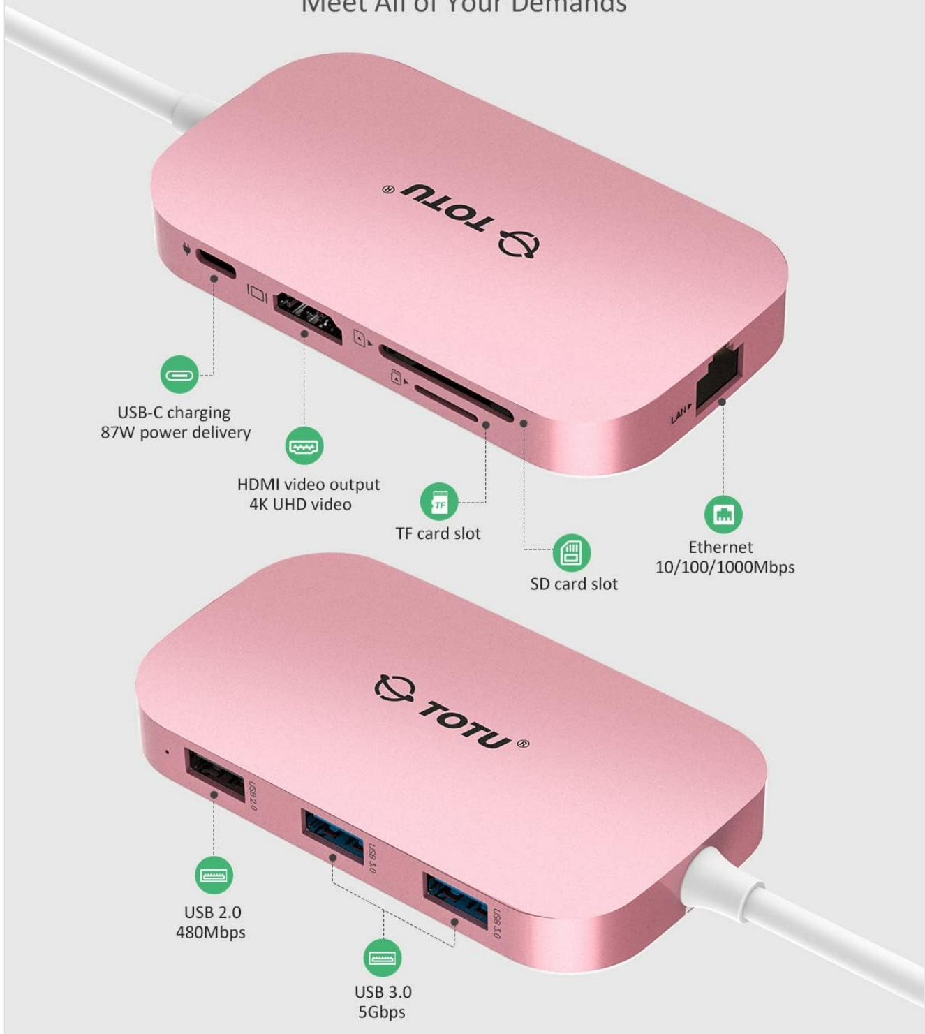
Figure 2.1: Overview of the TOTU USB-C Hub's 8-in-1 port configuration, including USB-C PD, HDMI, TF/SD card slots, Ethernet, USB 2.0, and USB 3.0 ports.
