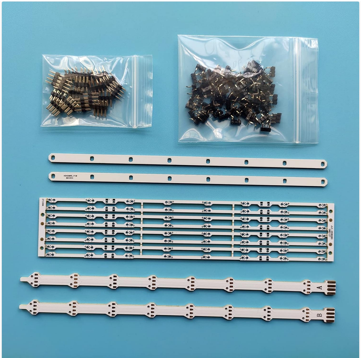
Image: A closer view of some of the smaller components, including different types of PCBs and bags of pin headers, essential for the cube's construction.
