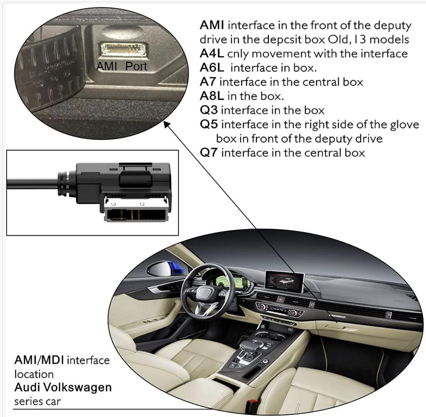
Image 4: Illustration of typical AMI/MDI interface locations in Audi and Volkswagen vehicles. Examples include AMI in the front of the glove box (Old, 13 models), A4L only movement with the interface, A6L in the box, A7 in the central box, A8L in the box, Q3 in the box, Q5 in the right side of the glove box, and Q7 in the central box.
