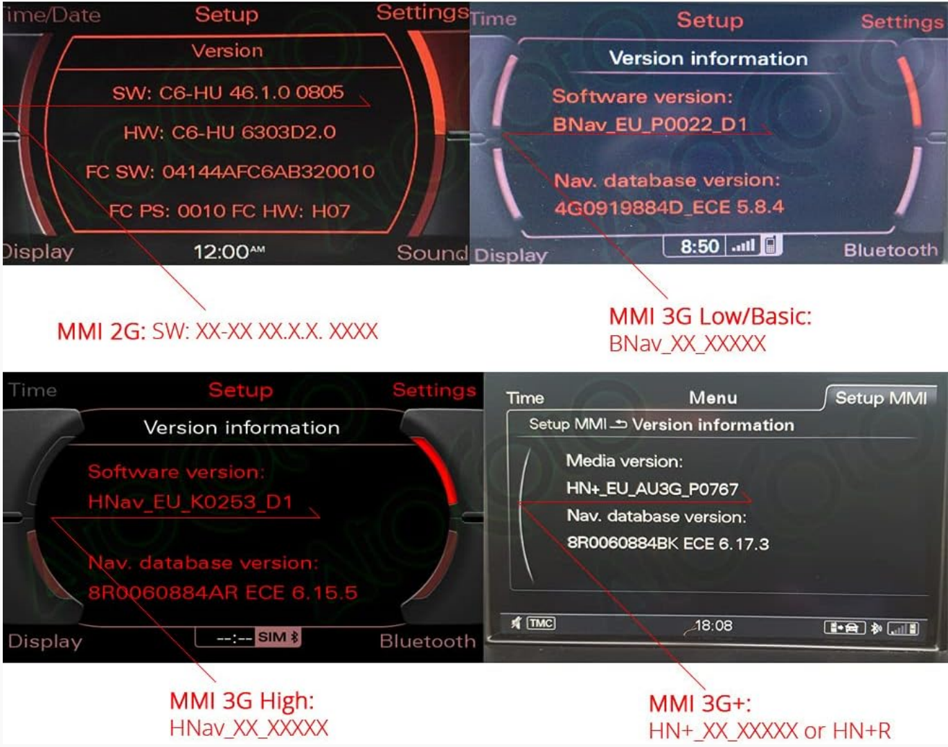
Image 6: Screenshots illustrating how to navigate the MMI system to identify whether it is an MMI 2G or MMI 3G system by checking the software version information.
