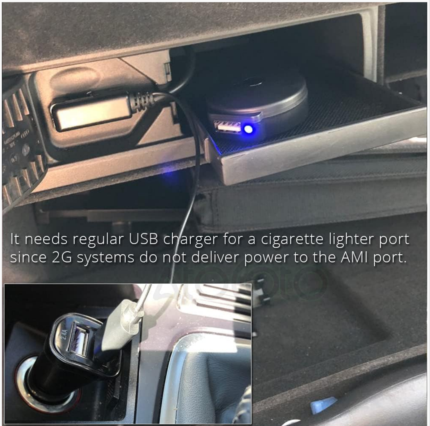
Image 7: The Bluetooth receiver connected to the AMI port inside a glove box, with its USB cable routed to a cigarette lighter for power. This setup is necessary as 2G systems do not provide power to the AMI port.
