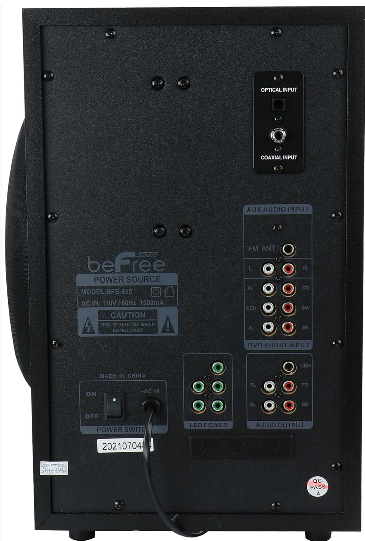
Image: Rear panel of the subwoofer, detailing the optical input, coaxial input, AUX audio input, FM antenna port, DVD audio input, LED power, audio output for satellite speakers, and power switch.
