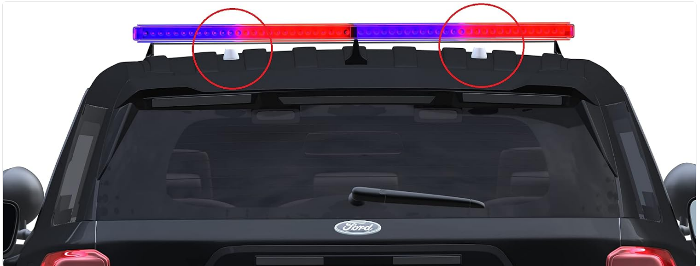
Image: Rear view of a vehicle demonstrating the Parsec antenna mounted on the roof. The antenna is strategically placed to allow for the installation of an LED light bar, showcasing its low-silhouette design. Red circles indicate the mounting points.
