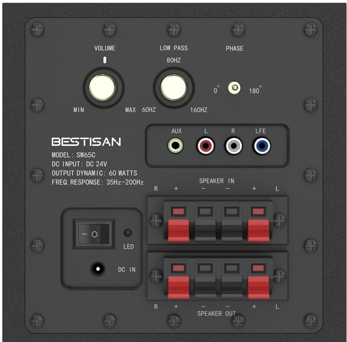
Image: Detailed view of the BESTISAN SW65C subwoofer's rear panel, showing all control knobs and input/output ports.
