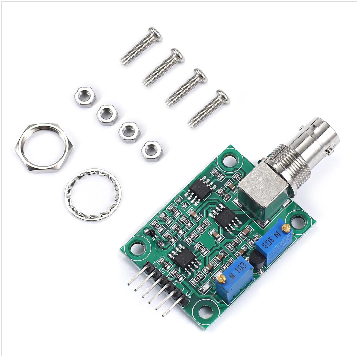
Image 2.2: Close-up of the sensor module and included mounting hardware (screws, nuts, washers).
