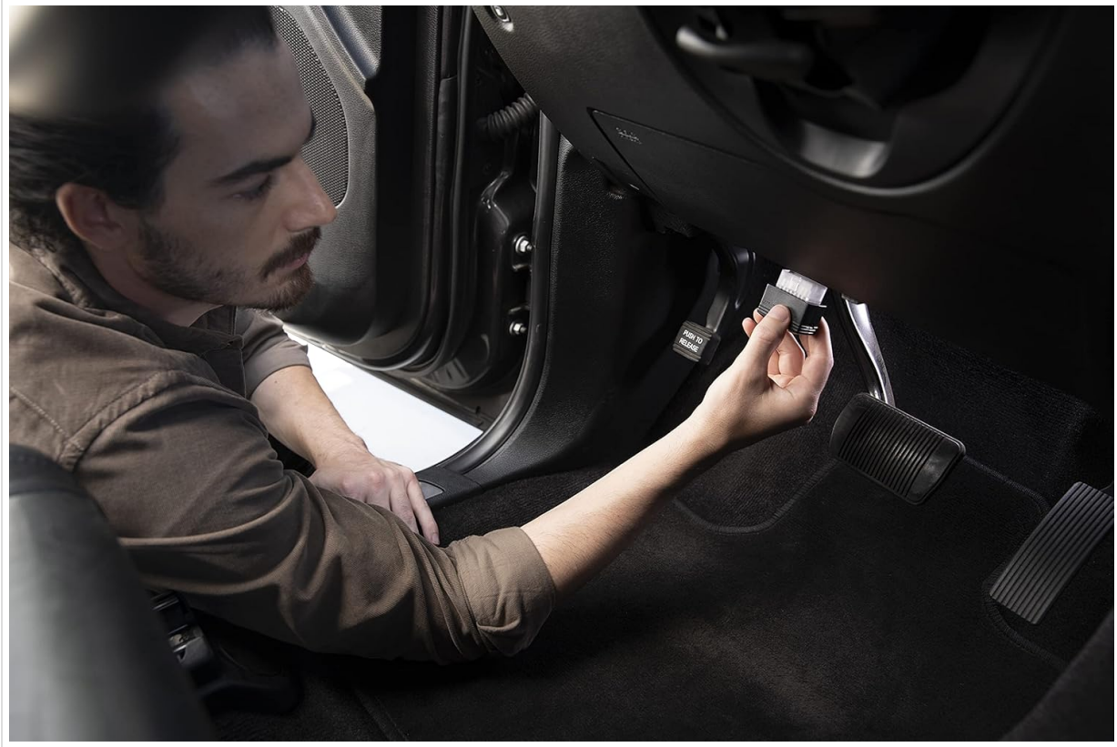
Image: A person is shown plugging the Innova 3215RS dongle into the OBD2 port, which is typically found beneath the steering wheel in most vehicles.
