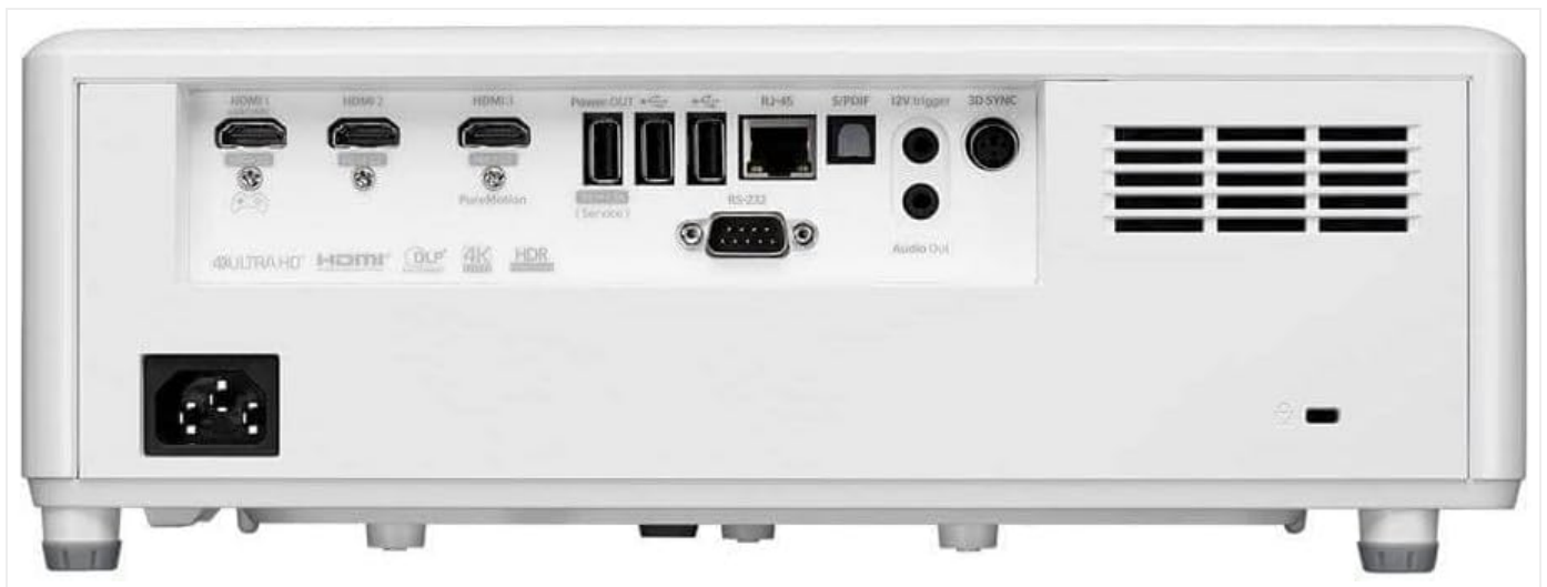
Figure 2.3: Rear panel of the projector, displaying various input and output ports including HDMI, USB, and audio connections.
