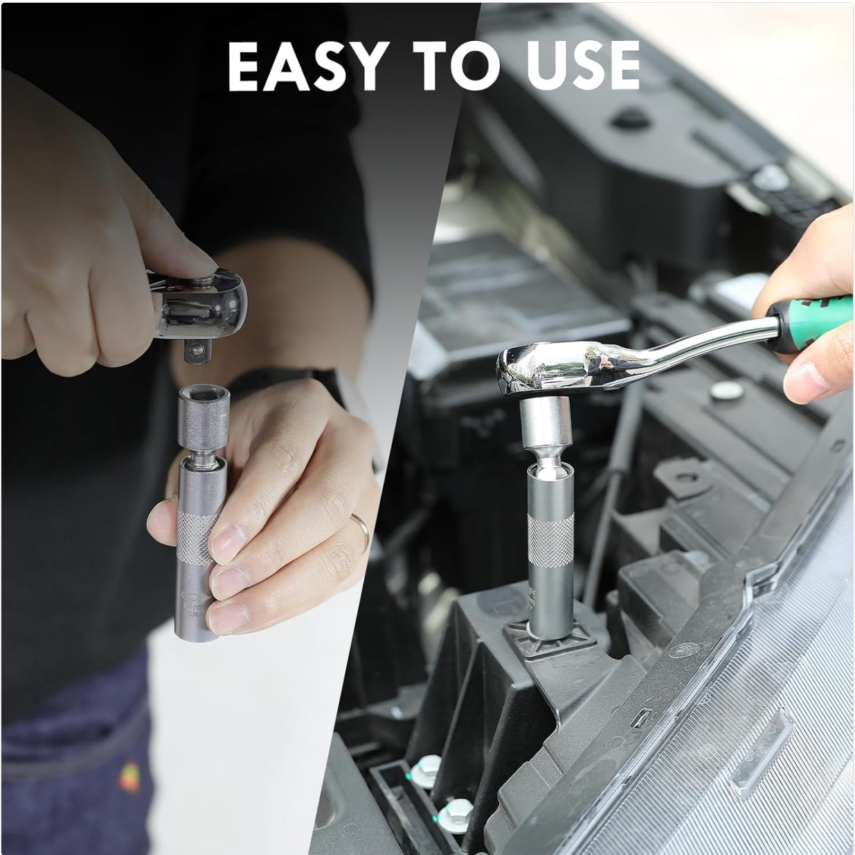
Image 4.1: Demonstrating how to attach the spark plug socket to a ratchet.
