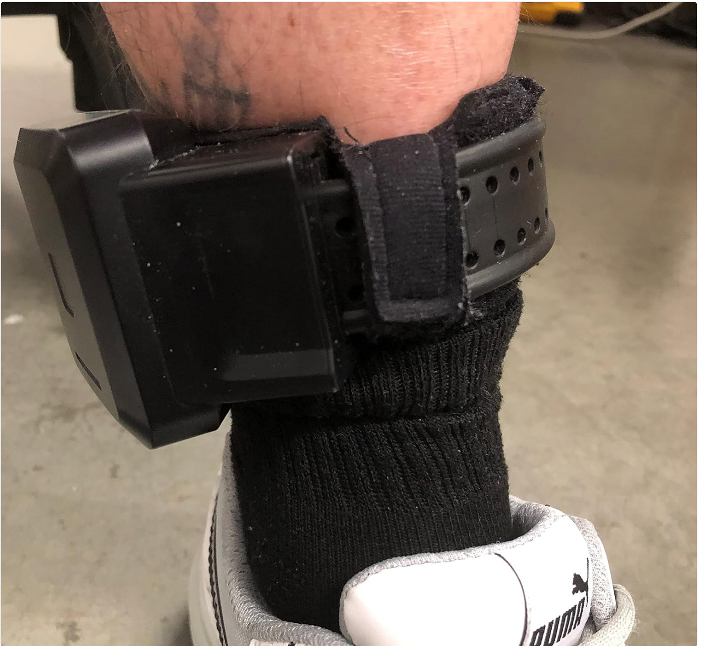
Image: The "Keep" strap maintaining the monitor's position while wearing a shoe.
