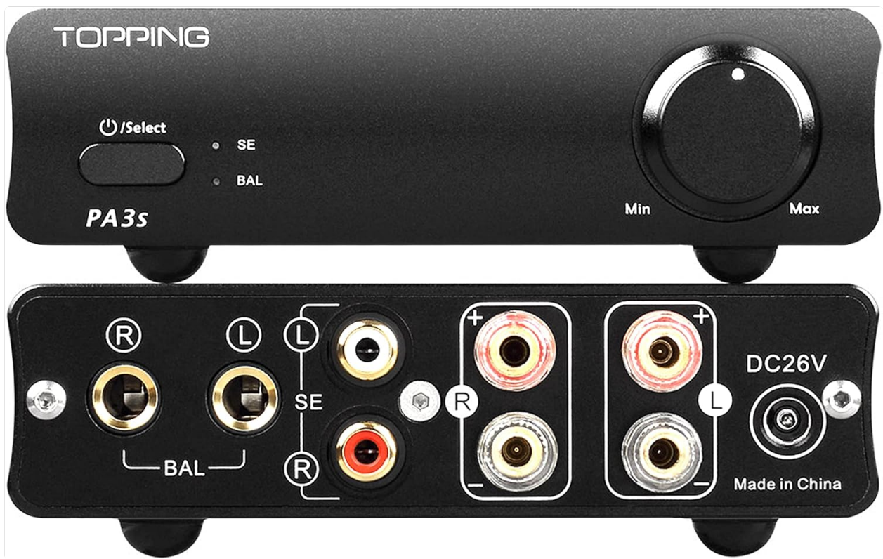
Image: Front panel showing power/select button and volume knob, and rear panel with input and output connections.
