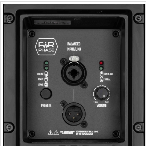
Figure 4.3: Close-up of the RCF Art 945-A control panel. This detailed image shows the Balanced Input/Link XLR connectors, the PRESETS button with LED indicators for LINEAR, BOOST, and STAGE modes, the VOLUME knob, and LED indicators for OVERLOAD and SIGNAL. A 'CAUTION' warning label is also visible.
