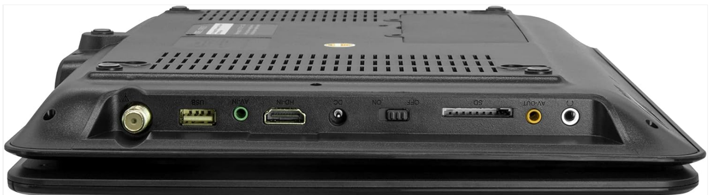
Image: Rear view of the player, showing the arrangement of connection ports.
