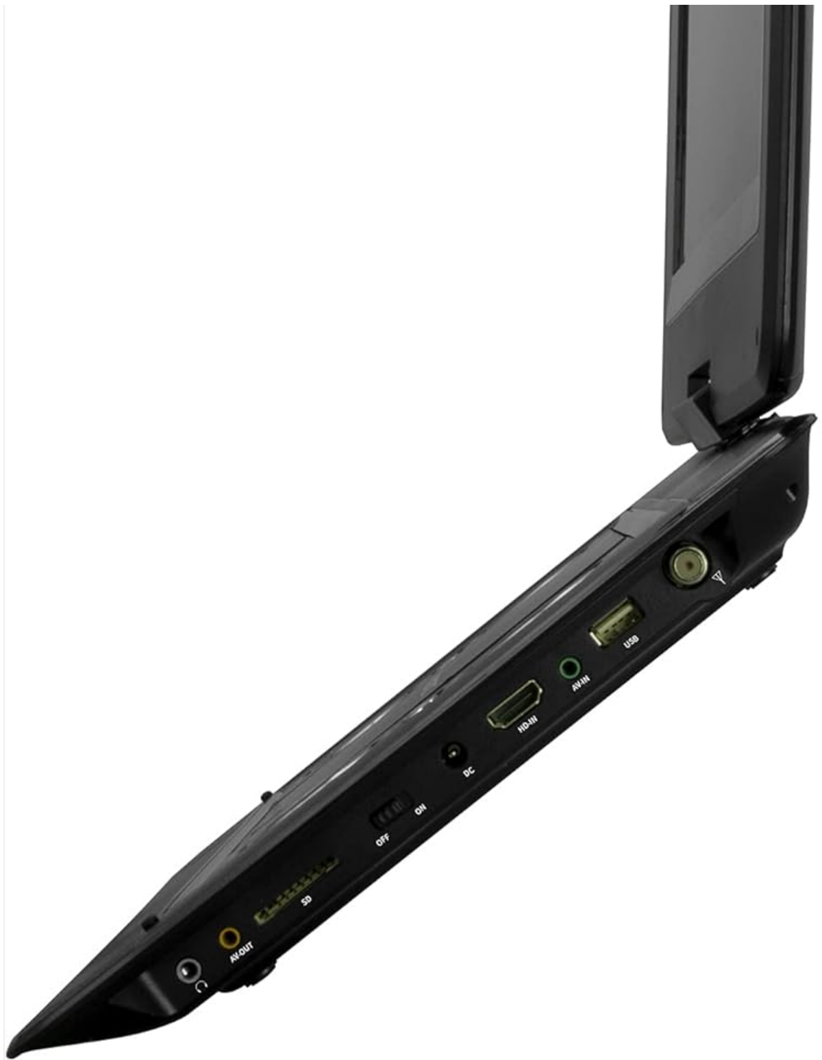
Image: Side view of the player, highlighting various input and output ports.
