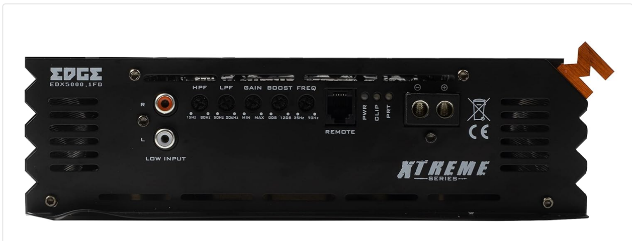
Image 4.2: Rear panel of the EDX5000.1FD-E0 amplifier, showing low-level inputs, crossover controls, gain, bass boost, and speaker output terminals.
