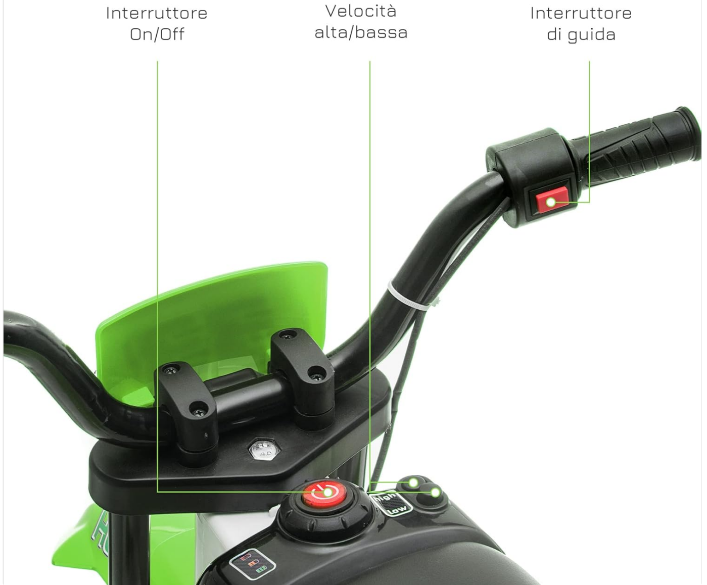
Image 4.1: Handlebar controls for the electric dirt bike.
