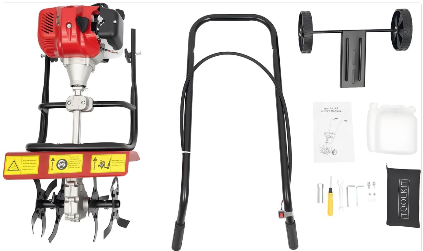
Figure 3.1: Tiller Components. This image displays all the parts included in the package, such as the main engine unit, handles, wheels, and toolkit, before assembly.
