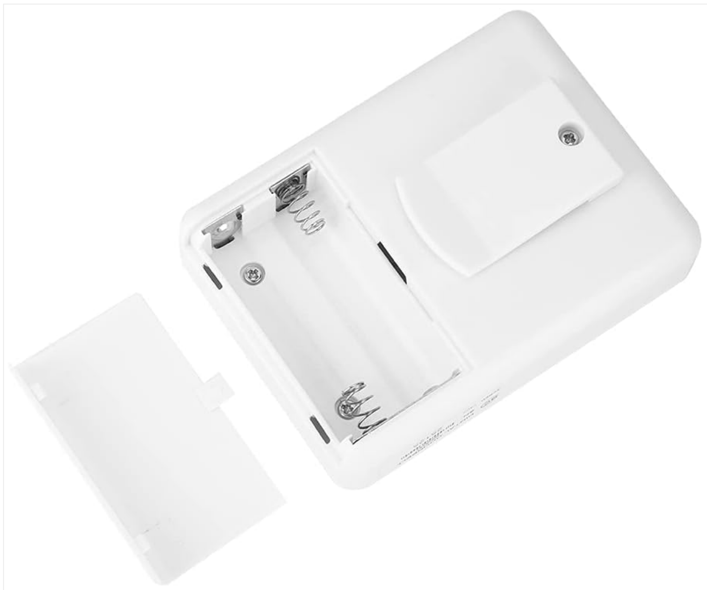
Figure 3.4: Receiver unit with battery compartment open.
