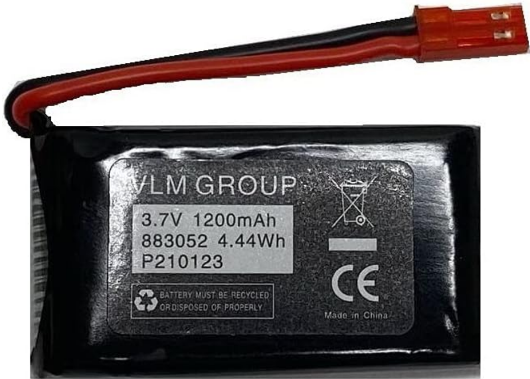
Figure 2.1: Close-up view of the VLM 3.7V 1200mAh battery, showing the label with specifications such as voltage, capacity, and manufacturing details. The label also includes recycling symbols and CE marking.
